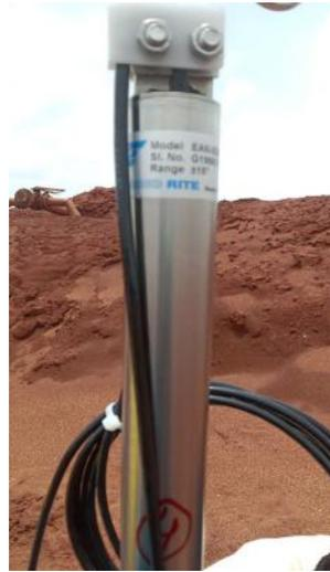
IPI being installed in red mud embankment area
